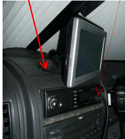
Added high-level mirror [to see vehicle travelling closer behind than can be seen in existing mirrors]
