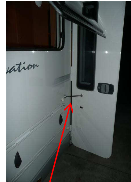
Added cabin hook to hold door at 90 degree position [to permit window to be opened whilst door held open]
