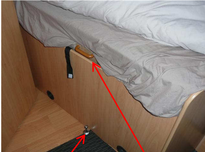
Added magnetic door stop [to hold bathroom door open when required]
