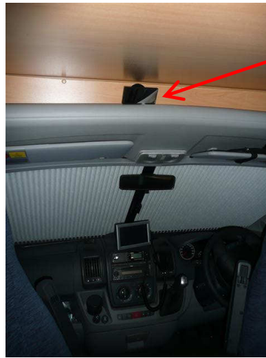
Added high-level mirror [to see vehicle travelling closer behind than can be seen in existing mirrors]
