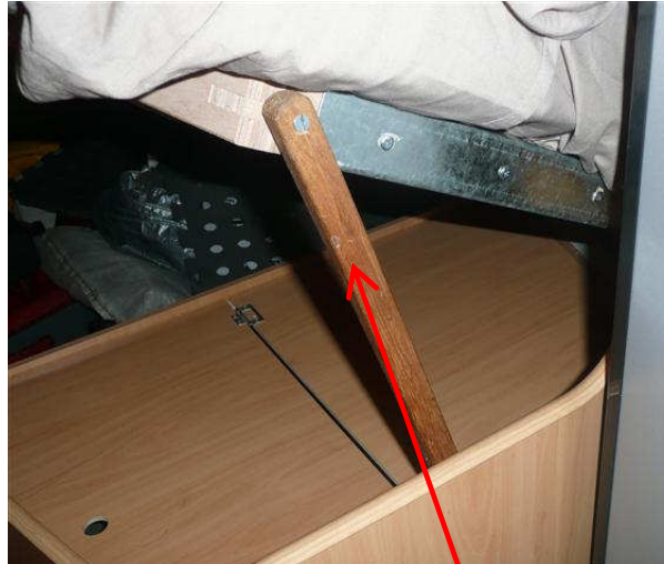
Added handle [to assist with lifting bed] NOTE: additional gaslift strut required to balance weight of doona, sheets & pillows
